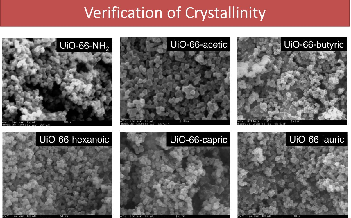
**SEM.** Analysis by scanning electron microscopy (SEM) reveals that the morphology of modified MOF particles remains unchanged by the PSM reaction.
