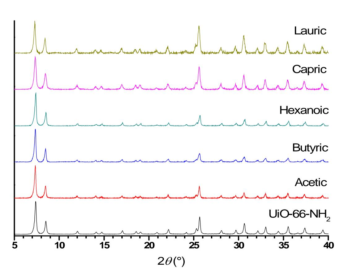
**PXRD.** Powder X-ray diffraction (PXRD) spectra indicate preservation of the crystalline structure of the MOF after the PSM reaction.
