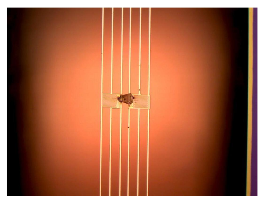
This is the next magnification at a magnification of 200X. This is the two wires and there is the bundle of wires that are making a bridge between the two suspended wires. One must use great precision to place this Geranium Telluride wires on the circuit board and leave the area without bumping into anything or breaking the wires on the circuit board.
