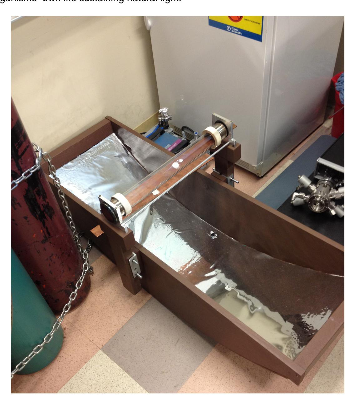
The copper plates are inside the tub that is at the middle of the half circle. There is aluminum on the halfcircle so the lighe bounces into the copper rods
