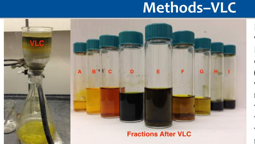
Nine fractions were created with varying parts of Hexane, Ethyl Acetate, and Methanol to create varying polarities (different compounds will move with different speed, which is related to their polarity). After first adding the crude extract to the packed VLC funnel, each fraction from least to most polar was run through.
