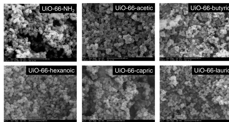
**SEM.** Analysis by scanning electron microscopy (SEM) reveals that the morphology of modified MOF particles remains unchanged by the PSM reaction.
