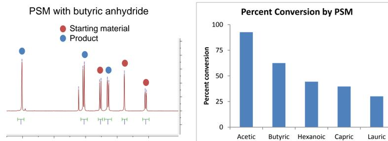
**NMR.** Analysis of the digested MOFs by nuclear magnetic resonance (NMR) spectroscopy allowed determination of PSM conversion efficiency by peak integration.
