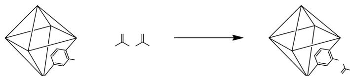
UiO-66-NH<sub>2</sub> powder (60 mg) was dispersed in CHCl<sub>3</sub> (2 mL) with 1 equivalent of the anhydride (acetic, butyric, hexanoic, capric, and lauric). The reagents were held at 55°C for 24 hrs. The resulting MOF precipitate was collected by centrifuge and washed with CHCl<sub>3</sub> and methanol.
