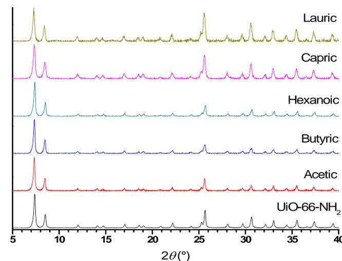
**PXRD.** Powder X-ray diffraction (PXRD) spectra indicate preservation of the crystalline structure of the MOF after the PSM reaction.
