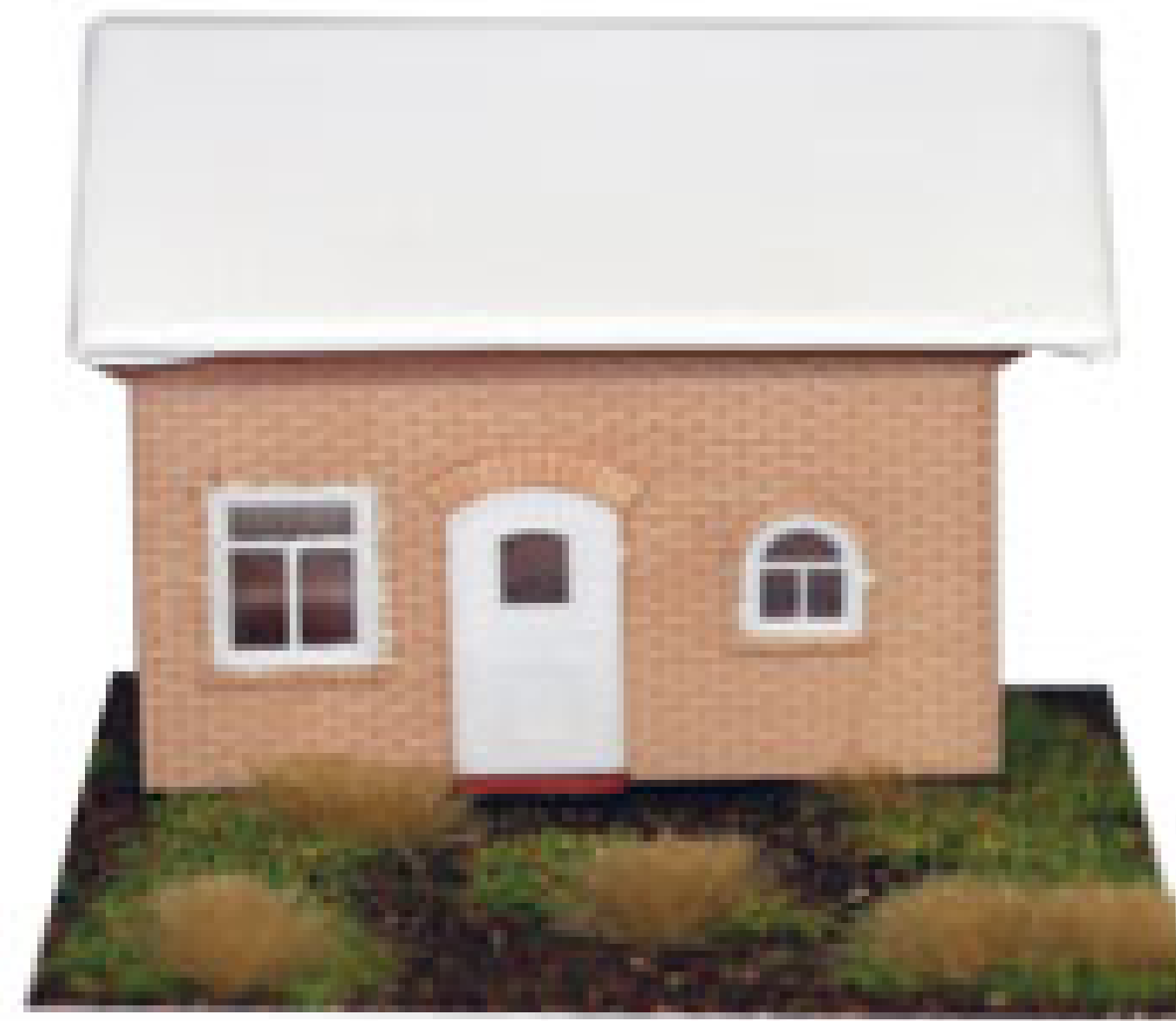
Figure 3 - A practical model house that could be used as a scale model to test effectiveness of hydrogel on constructions.
