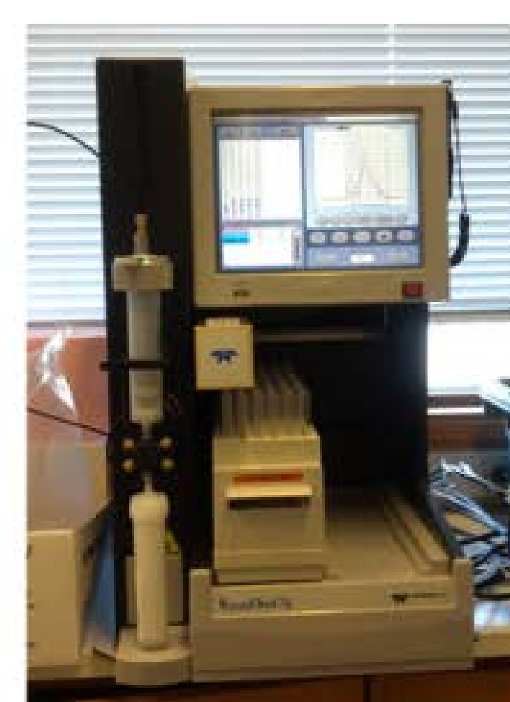
Auto Column: Silica Purification Column system
