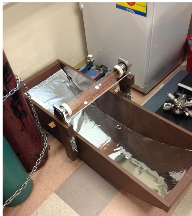
The copper plates are inside the tub that is at the middle of the half circle. There is aluminum on the halfcircle so the light bounces into the copper rods
