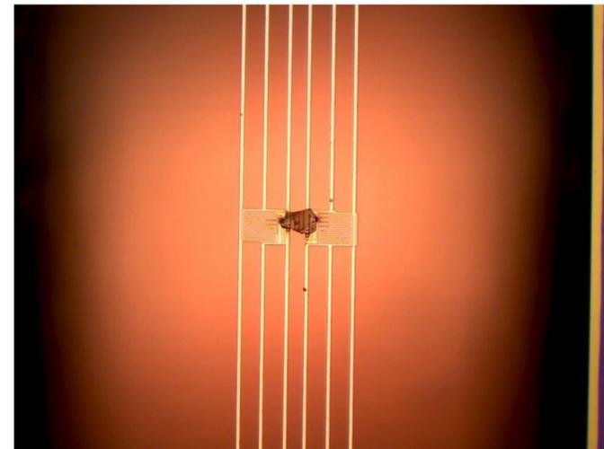
This is the next magnification at a magnification of 200X. This is the two wires and there is the bundle of wires that are making a bridge between the two suspended wires. One must use great precision to place this Geranium Telluride wires on the circuit board and leave the area without bumping into anything or breaking the wires on the circuit board.
