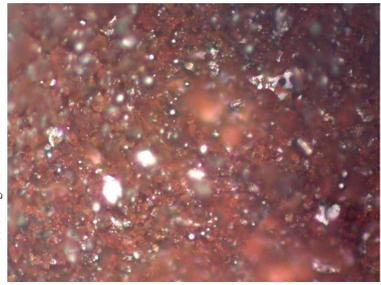
A silicon-germanium alloy placed on a silicon plate heated at 900 C and 1000 C for 1 and 3 hours. Exposed to hydrogen and argon at a 1 to 1 ratio. The melting point is 1380.2 C
