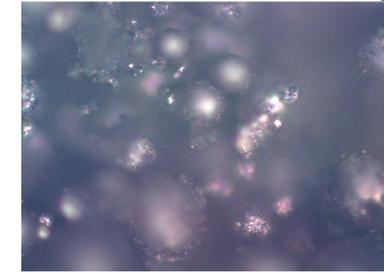
A bismuth powder on a silicon plate heated between 240-270 C at intervals of 10. Heated for 1 -3 hours. Exposed to hydrogen and argon at a 1 to 1 ratio.. The melting point is 271.5 C
