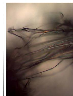
Higher amounts of nanowires were found at this temperature. This suggests that the starting temperature for nanowire growth is between 245 C and 248 C
