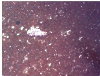
Also, no visible change when viewed with light microscope. The most valid reason was that the temperature was too low compared to the melting temperature
