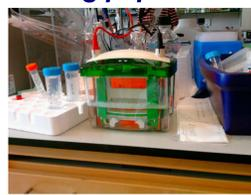
A current runs through the gel cassette and separates the proteins based on size. The dye from the samples will bleed onto the blotting paper.
