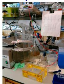
A current passes through the agarose gel and separates nucleic acids based on size.
