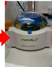
Cultures are spun down in a centrifuge to isolate the bacterial pellet containing DNA.
