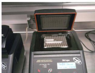
DNA samples are loaded into PCR tubes and placed in a PCR machine for 2 1/2 hours.
