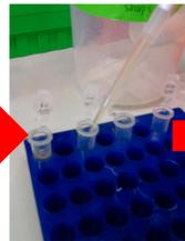
The media is transferred to smaller tubes and centrifuged.
